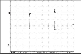
Figure 5: Output voltage response to step-change in load current (50%-75%-50% of lout(max);  $dI/dt = 0.1A/\mu s$ ). Load cap:  $1\mu F$  ceramic cap. Ch 1: Vout, Ch 2: Jout
