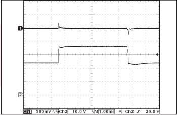
Figure 6: Output voltage response to step-change in input voltage (nominal to maximum), at full load current. Load cap: 15µF tantalum capacitor and 1uF ceramic cap. Ch 1: Vout, Ch 2: Vin.
