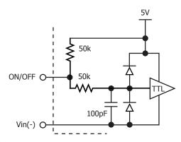
Figure B: Internal ON/OFF pin circuitry
