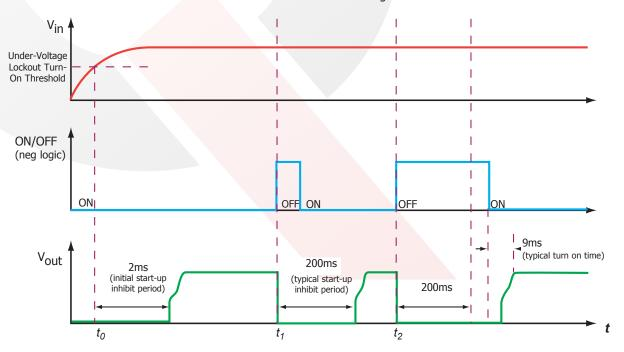
Figure E: Startup Inhibit Period (turn-on time not to scale)
