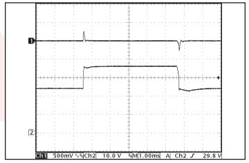
Figure 6: Output voltage response to step-change in input voltage (nominal to maximum), at full load current. Load cap:  $15\mu F$  tantalum capacitor and 1uF ceramic cap. Ch 1: Vout, Ch 2: Vin.
