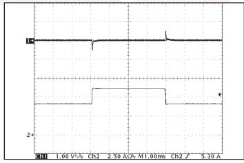
Figure 5: Output voltage response to step-change in load current (50%-75%-50% of lout(max);  $dI/dt = 0.1A/\mu s$ ). Load cap:  $15\mu F$  tantalum cap and  $1\mu F$  ceramic cap. Ch 1: Vout, Ch 2: Iout.
